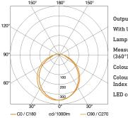
Output With lamp Yes, STEINEL LED system LED cannot be replaced Measured luminos flux (360°) 576 lm 3000 K Colour temperature
